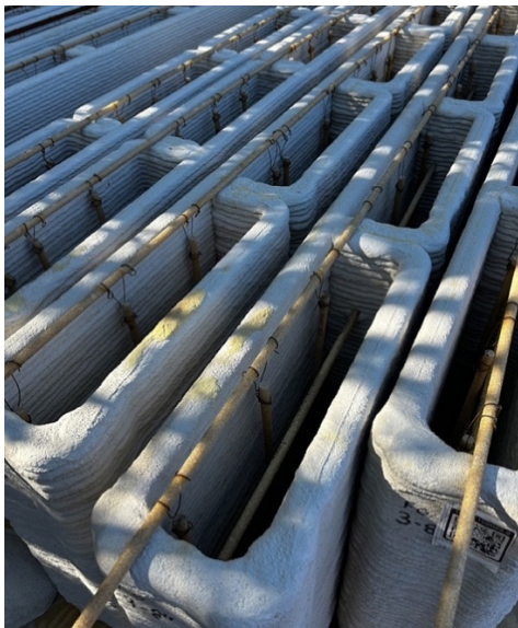
Figure 2C: 3D-printed component with fiberglass reinforcement
